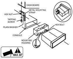
CAUTION: DO NOT PLACE THE UNIT OVER THE MAXIMUM INSTALLATION ANGLE OF 30°. OTHERWISE, THE UNIT MAY NOT WORK PROPERLY.
